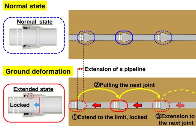
Figure 3. Behavior of a chain structure pipeline
