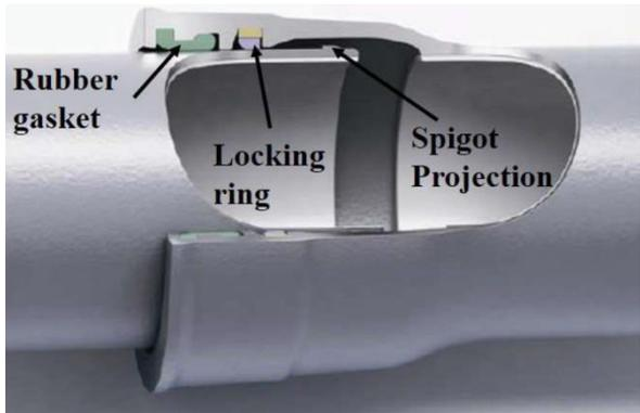
Figure 1. Cut-away view of a GX-type joint
